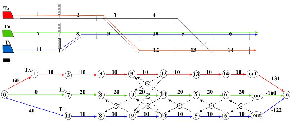
Each alternative pair is used to order two trains on a block section
